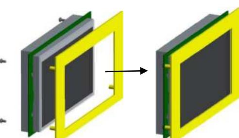
The touch TP is physically pasted on the sheet metal shell. In the cabinet design, the TP should not be suspended to prevent falling off. It is suggested that a buffer foam with a width of less than 5mm can be added at the front edge of touch TP (too large to block the LCD effective display area) to pad between the cabinet and the touch TP to form appropriate extrusion, so as to achieve the auxiliary reinforcement effect of touch TP.
