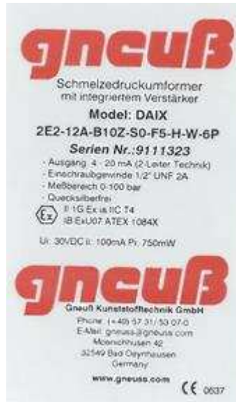
Fig. 1 The Type-label for a device with Ex approval This kind of type-label must not be removed from the device!
